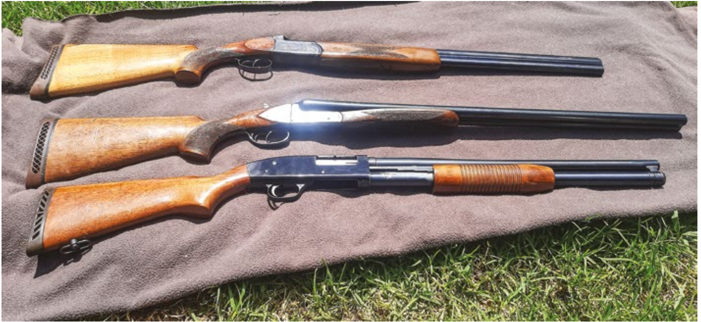
Three types of shotguns: over-and-under (top), side-by-side (middle) and a pump-action (bottom).
